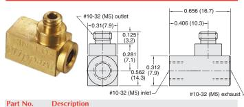
MEV-2 MEV-2-M5 Poppet Type Quick Exhaust Valve, #10-32 Poppet Type Quick Exhaust Valve, M5
